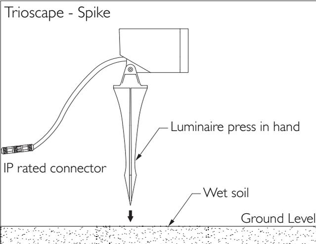
Please ensure that the wires are connected to the right polarity. [Phase, Neutral, Earth] and the luminaire must be earthed ( Class I.)
