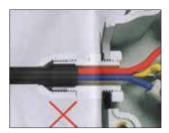
The best and easiest ways to prevent the water filtration are by IP rated connectors
